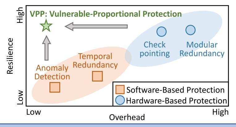
**Insight & Solution**: exploit the *inherent resiliency variations* in autonomous machine system to conduct *vulnerable-proportional protection (VPP)*
