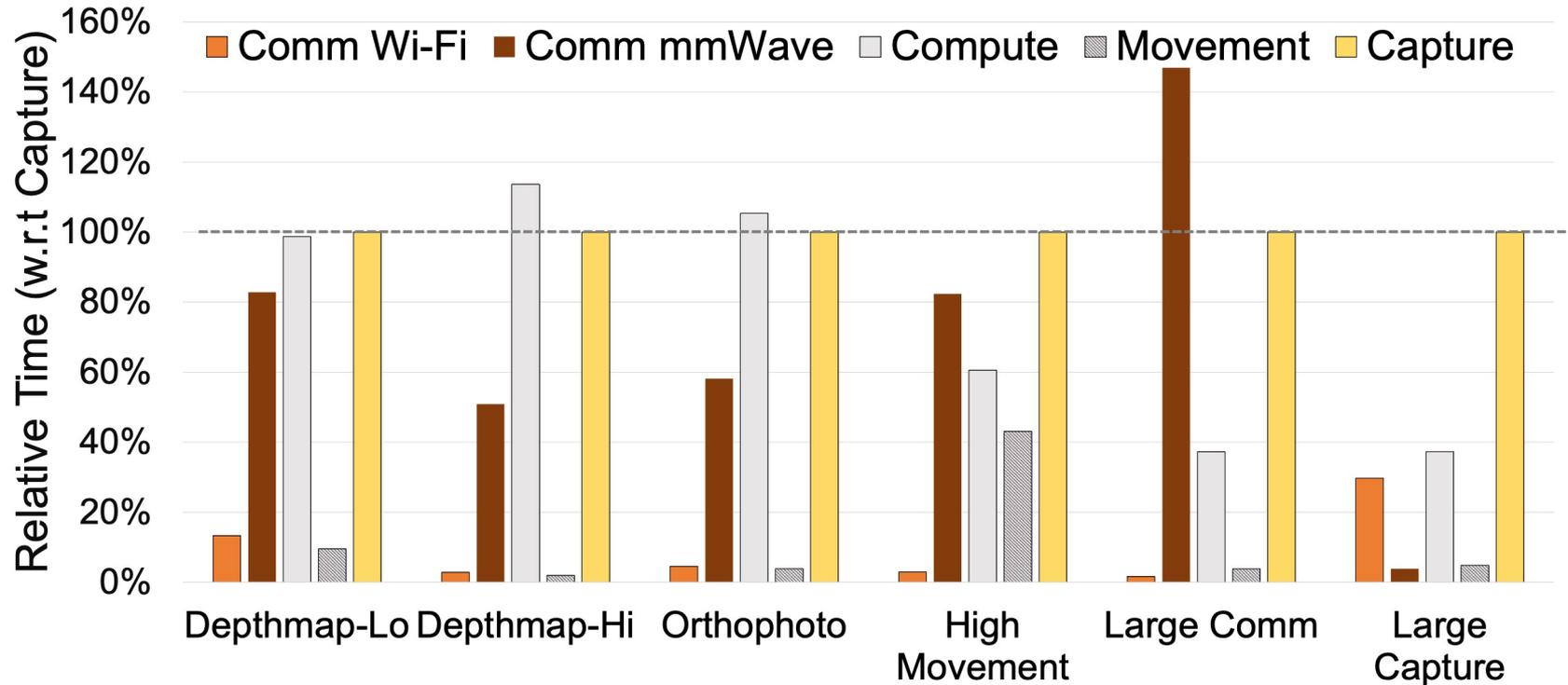
Time spent on each subtask (normalized to capture); mmWave's contribution to communication in DynaaDCP.
