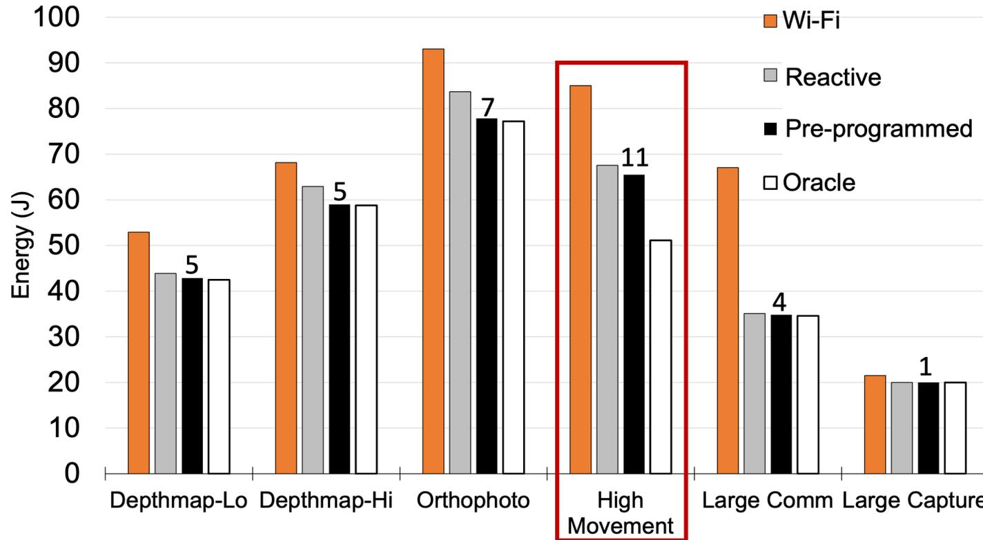
Despite multiple near ↔ far transits (numbers on graphs), total energy consumption reduces due to shorter flight times.
