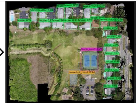
Output of the Orthophoto and YOLOv4 object detection.
