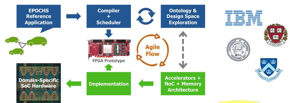
**Agile methodology** to quickly design and implement an <u>easily programmed</u> domain-specific SoC for real-time cognitive decision engines in connected vehicles
