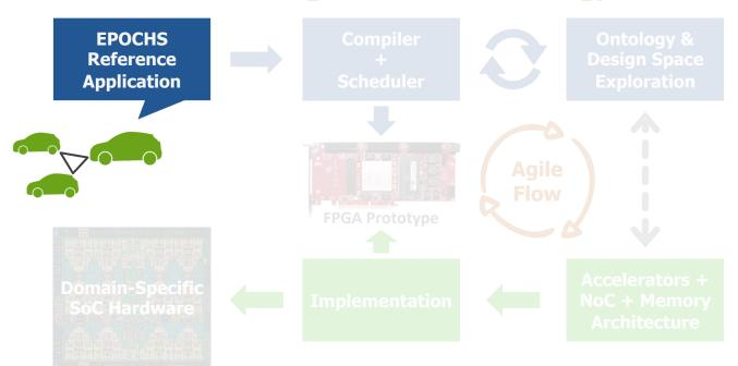
**Agile methodology** to quickly design and implement an easily programmed domain-specific SoC for real-time cognitive decision engines in connected vehicles
